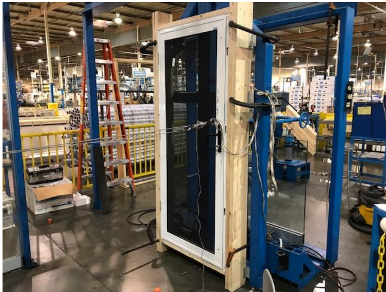
Photo No. 2 AAMA 1304 center pull at lock
