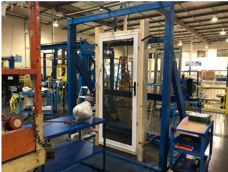
Photo No. 4 AS 5041 impact setup
