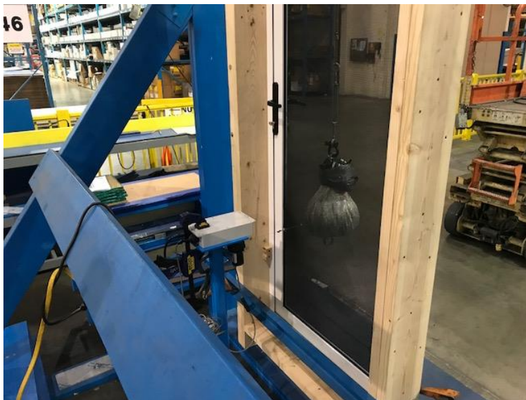
Photo No. 10 AS 5041 specimen interior after impact #5
